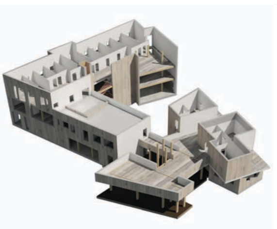
2nd floor CLT panels-walls
